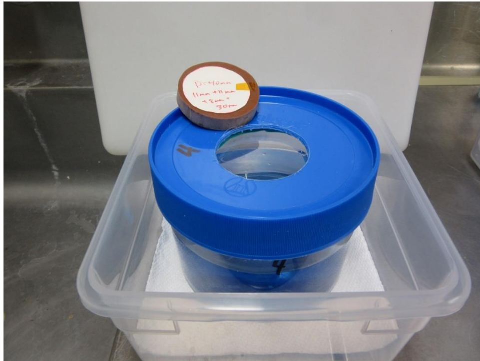
Figure 63: Phantom with outer lid on. There is a 40 mm diameter paper disk taped to the solid water plug. During use, the radiochromic film was taped to the solid water plug in the same manner.
