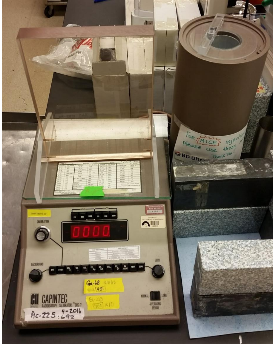
Figure 7: Shown is the dose calibrator used in these experiments. The readout module has the LED digits, range buttons and potentiometers for adjustment. The ionization chamber is the cylinder on the right side of photo.
