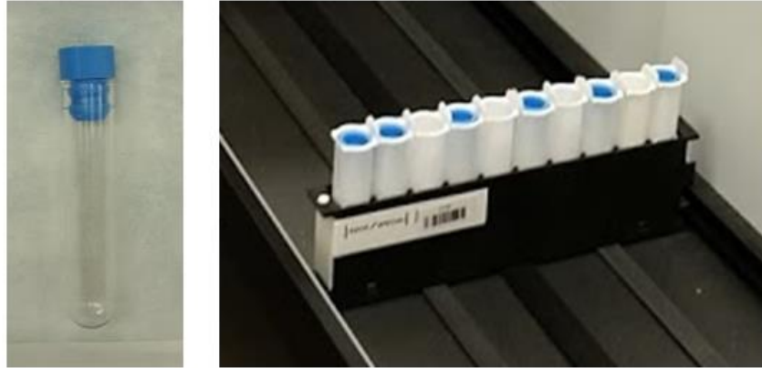
Figure 12: PerkinElmer sample vial (left). Vials in rack ready for counting in Wizard 2 counting system.
