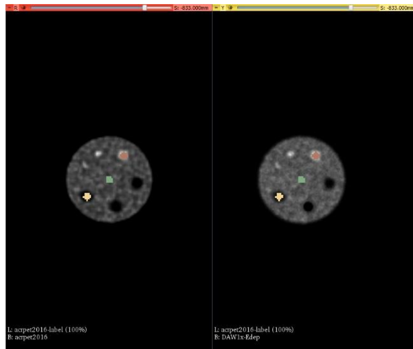
Figure 58: F-18 PET (left) and Y-90 Energy Deposited (right) and with spherical volumes of interest (VOIs) colored yellow, green, and red.
