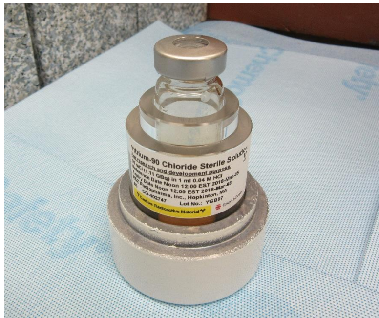
Figure 69: 10 mL P6 vial containing 30 mCi of Y-90 yttrium chloride in 1 mL volume.
