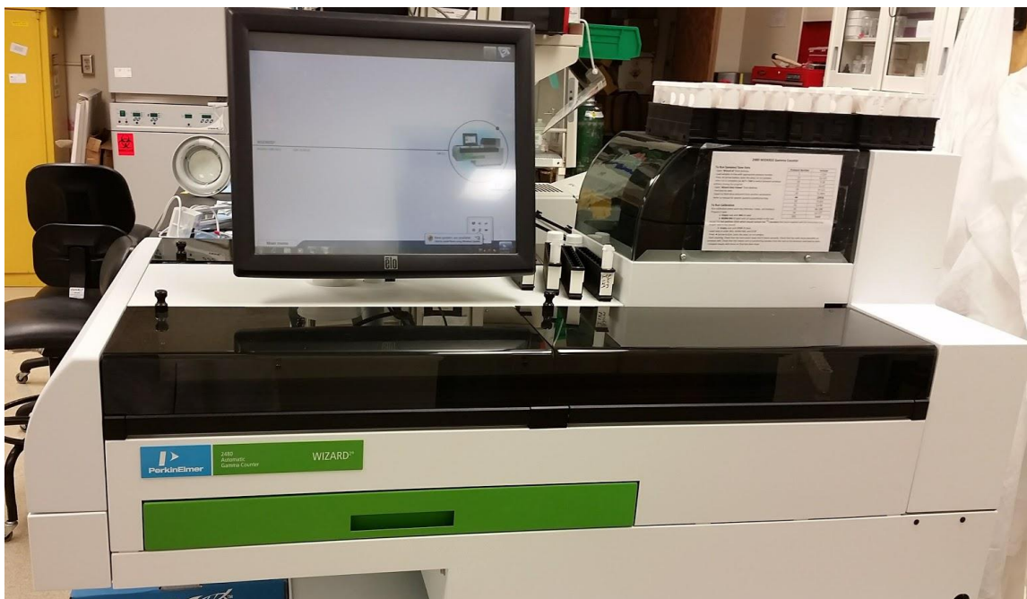
Figure 9: PerkinElmer "Wizard 2 " model 2480 automatic gamma counter.
